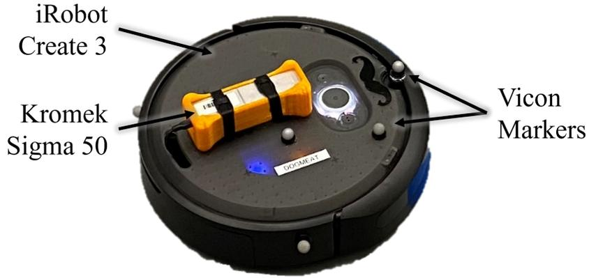
Figure 4.7: Robot to take measurements.
